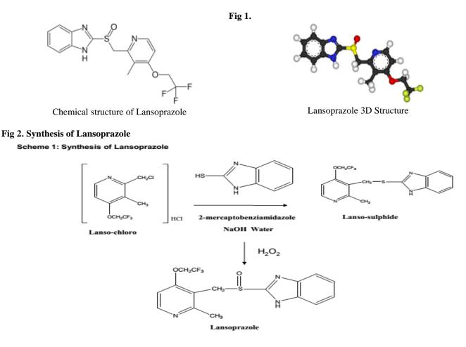
Fig 2: synthesis of Lansoprazole
